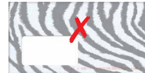
Avoid bleed printing into the coding area, the clear zone and coding area must be free of printing and lettering
